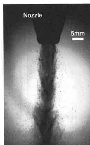
Fig.8 Snapshot of steam-water mixture.
